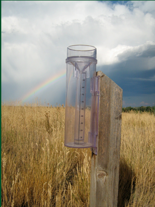
4-inch diameter High capacity rain gauges
