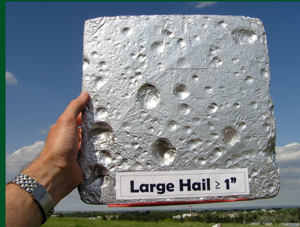
Aluminum foil-wrapped Styrofoam hail pads
