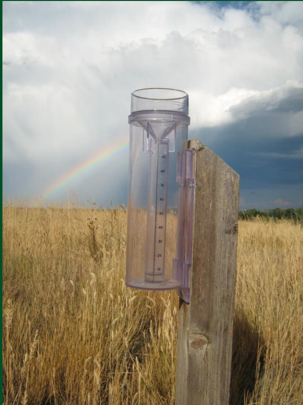
4-inch diameter High capacity rain gauges
