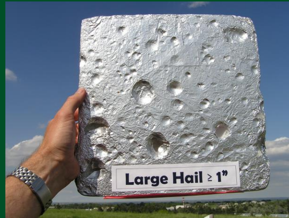
Aluminum foil-wrapped Styrofoam hail pads
