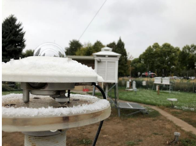
The first dusting of snow on the pyranometer* on October 10. Photo from Noah Newman
