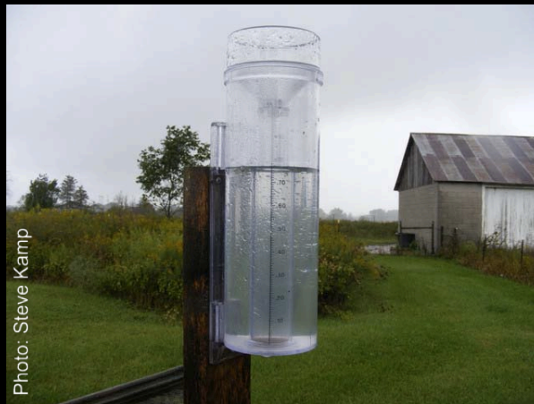
4-inch diameter High capacity rain gauges
