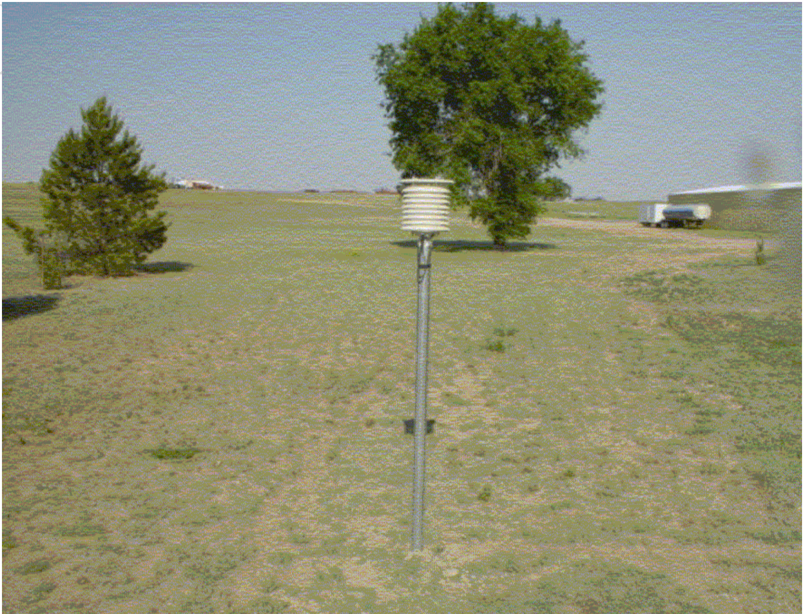
Maximum-minimum temperature sensor (MMTS) installation near Lindon, Colorado.
