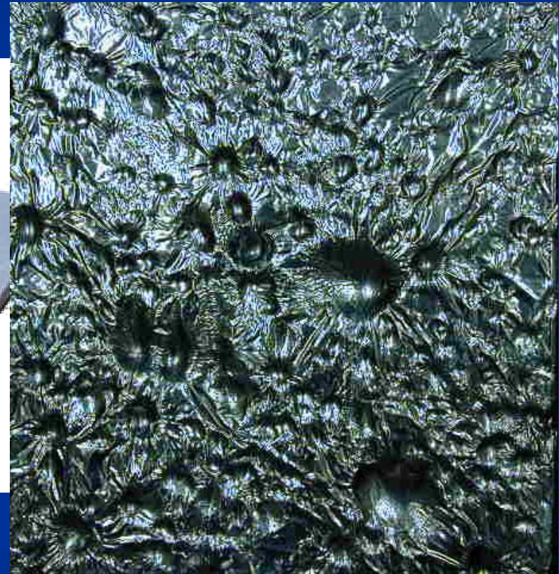
Damaged Hail Pad
