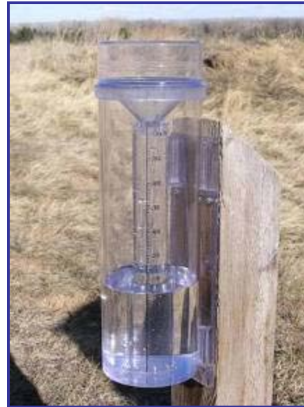
4-inch diameter high capacity rain gauges
