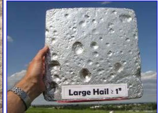
Aluminum foil-wrapped Styrofoam hail pads
